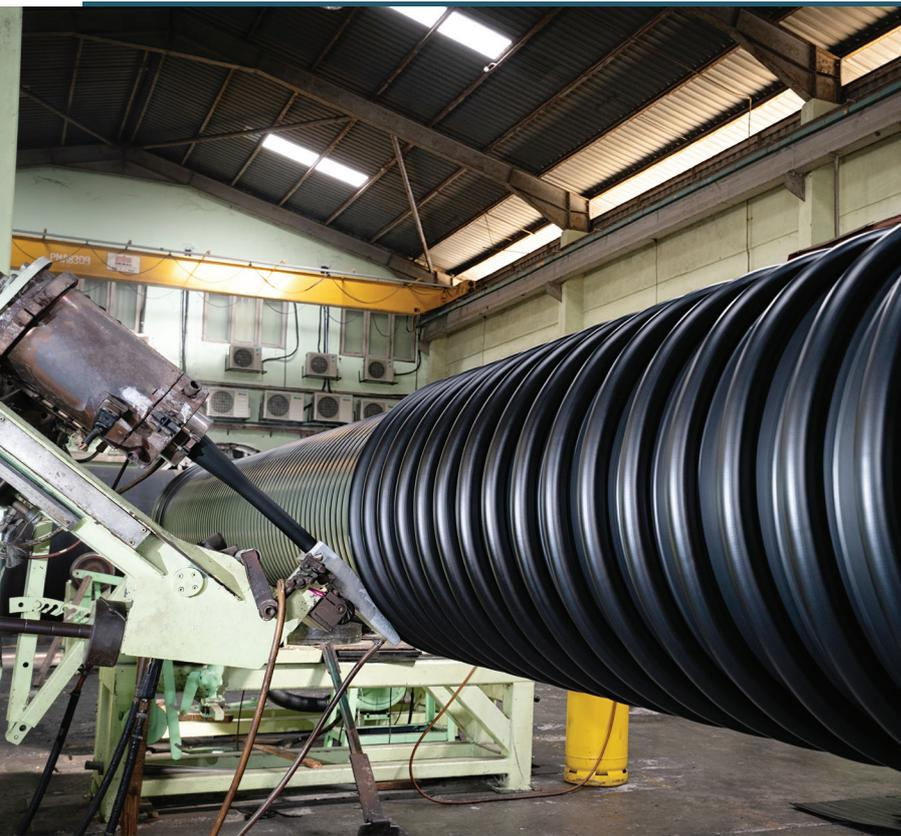
Spiral PE pipe are manufactured from weather resistant Polyethylene using a unique process by which a specially designed extruded profile strip is spirally wound over a pre-heated and revolving mandrel. Overlap on the edge is fused homogeneously together while it is in the hot plastic state, producing a smooth internal surface. The profile wall thickness is designed according to the ring stiffness required to withstand the loading on the pipe.
